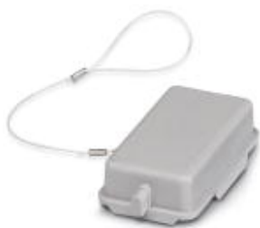
Protective cover B10, for single locking latch, protective cover material: PA, height: 18.5 mm, seal: no, With lanyard, diameter of retaining cord eyelet: 30 mm
