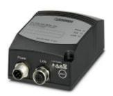
WLAN Ethernet port adapter, client, WLAN 802.11 a/n, 5.15 ... 5.25 GHz frequency, IP65, connections: M12 for 9 ... 30 V DC, M12 for LAN, autocrossing, PROFINET and PROFIsafe-compatible, web-based management, 802.11i, WPA2, WPA-PSK, WEP, TKIP, AES, integrated antenna
