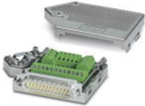
D-SUB connector, 25-pos., male connector, one cable entry < 35°, universal type for all systems, pin assignment: 1, 2, 3, ..., 24, 25 to screw connection terminal block
