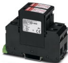
Surge protective device, two channel with remote indicator contact for 120/240 V split phase AC, 3-wire.
