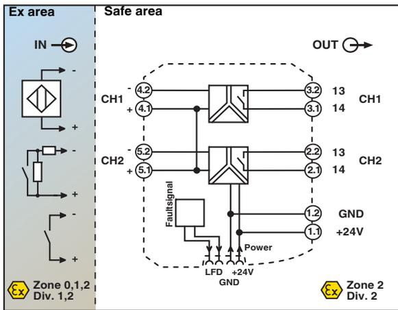
Figure 1 Basic circuit diagram with connection terminal blocks
