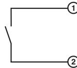
Figure 5 Switch contact with open circuit
