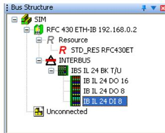
Figure 7-3 Complete bus configuration for the example project
