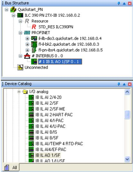
Figure 4-12 Device inserted (here: IB IL AO 1/SF)
