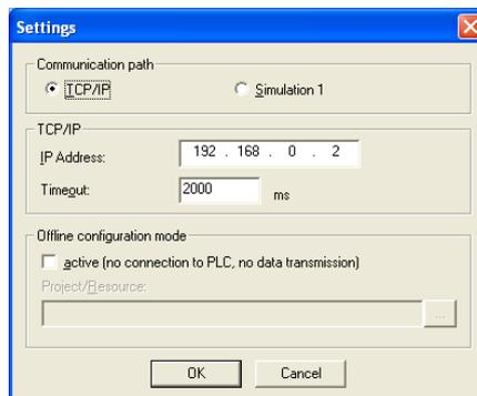
Figure C-7 Specifying the IP address of the controller
