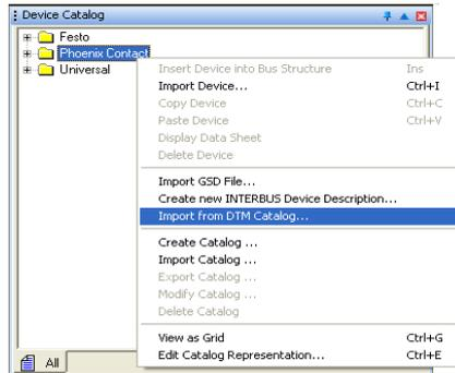
Figure 3-31 Integrating DTMs into the device catalog
