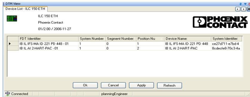
Figure 3-40 DTM functions: Controller device list
