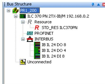
Figure A-8 Manually adapted bus configuration with new controller
