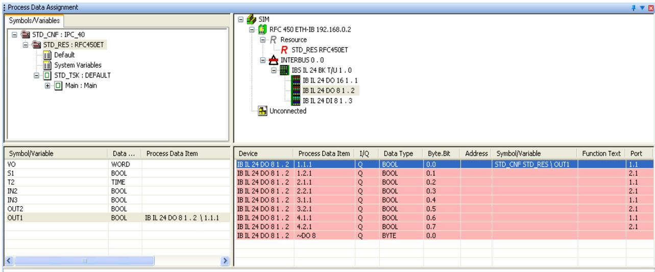
Figure 4-21 Process data item 1.1.1 assigned to variable OUT1
