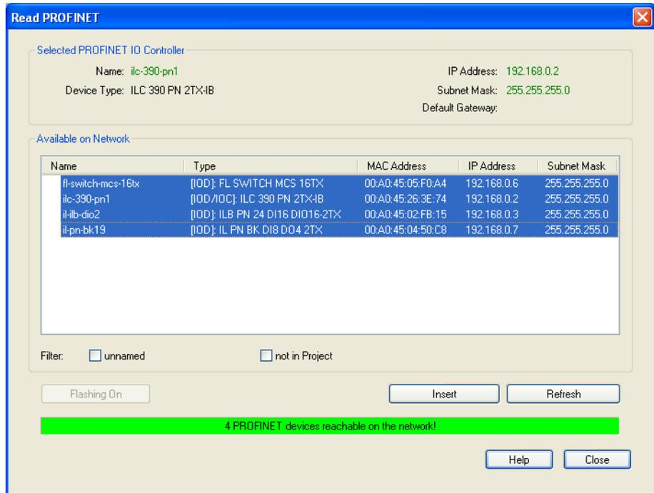
Figure 4-34 Connected and selected PROFINET IO devices for the project; PROFINET device names and IP addresses are already present
