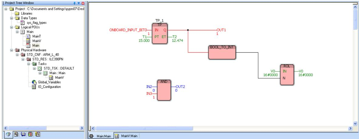
Figure 4-62 Variables in debug mode: Program variables
