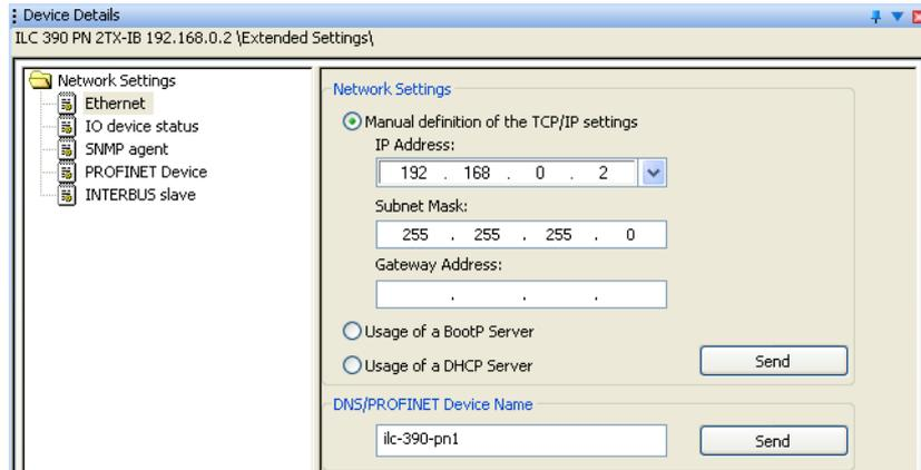
Figure 4-28 IP address of the PROFINET IO controller
