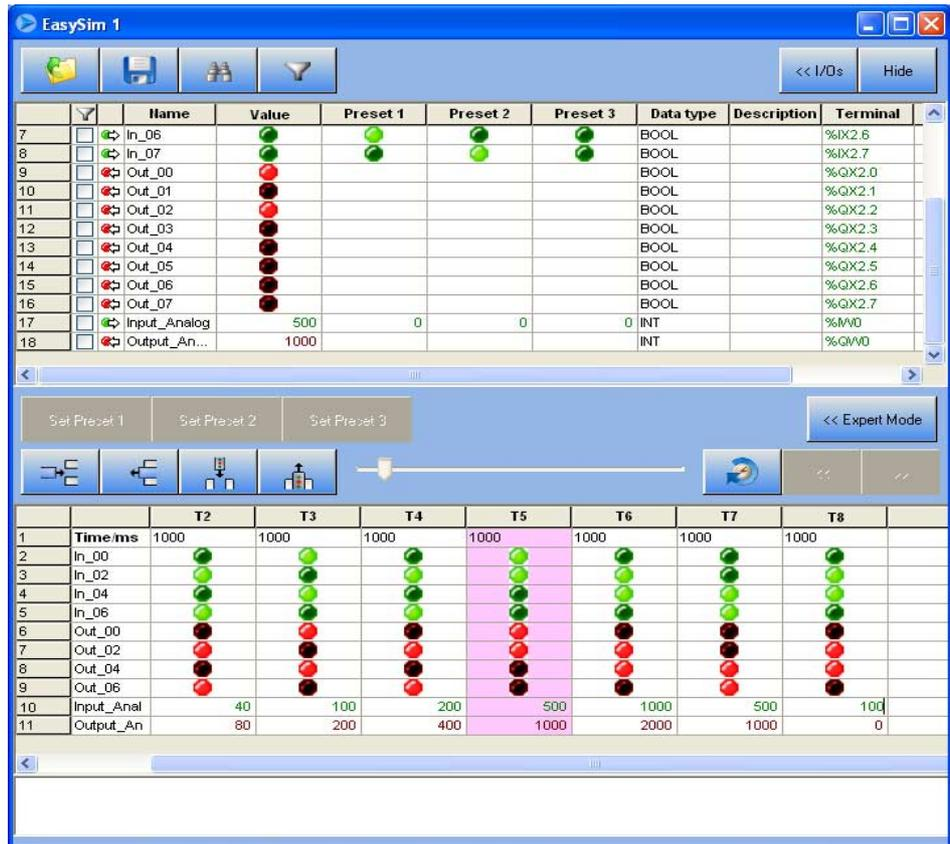
Figure 4-56 EasySim simulation: I/O view - Expert mode
