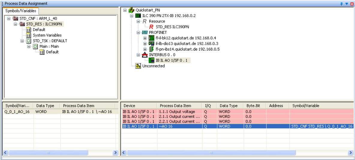
Figure 4-19 Variable generated for process data item "~AO 16"
