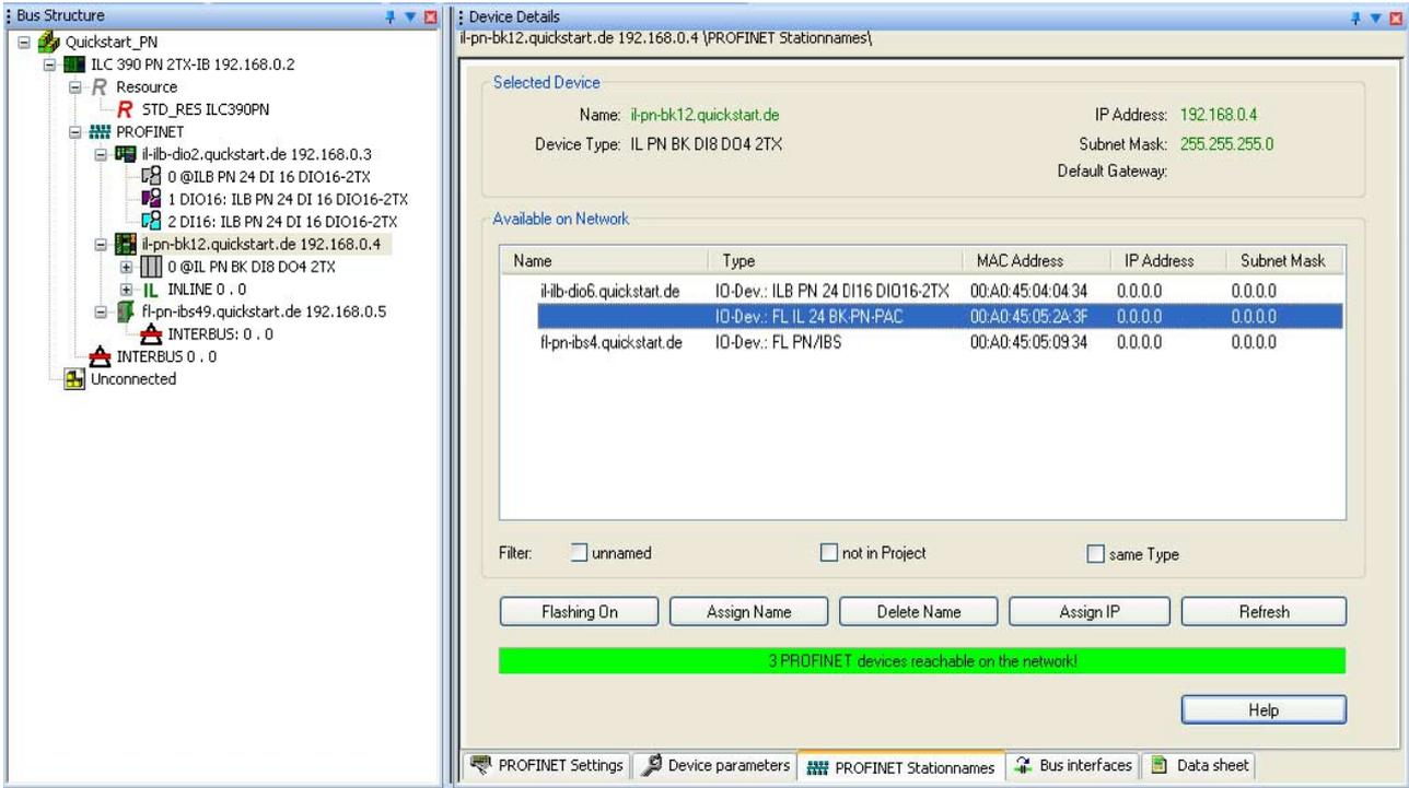
Figure 4-39 Assigning the PROFINET device name
