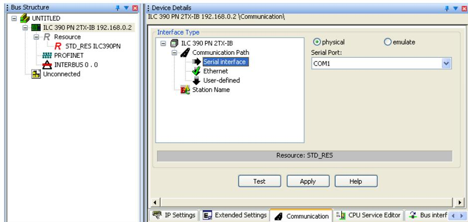
Figure 4-30 Setting the communication path
