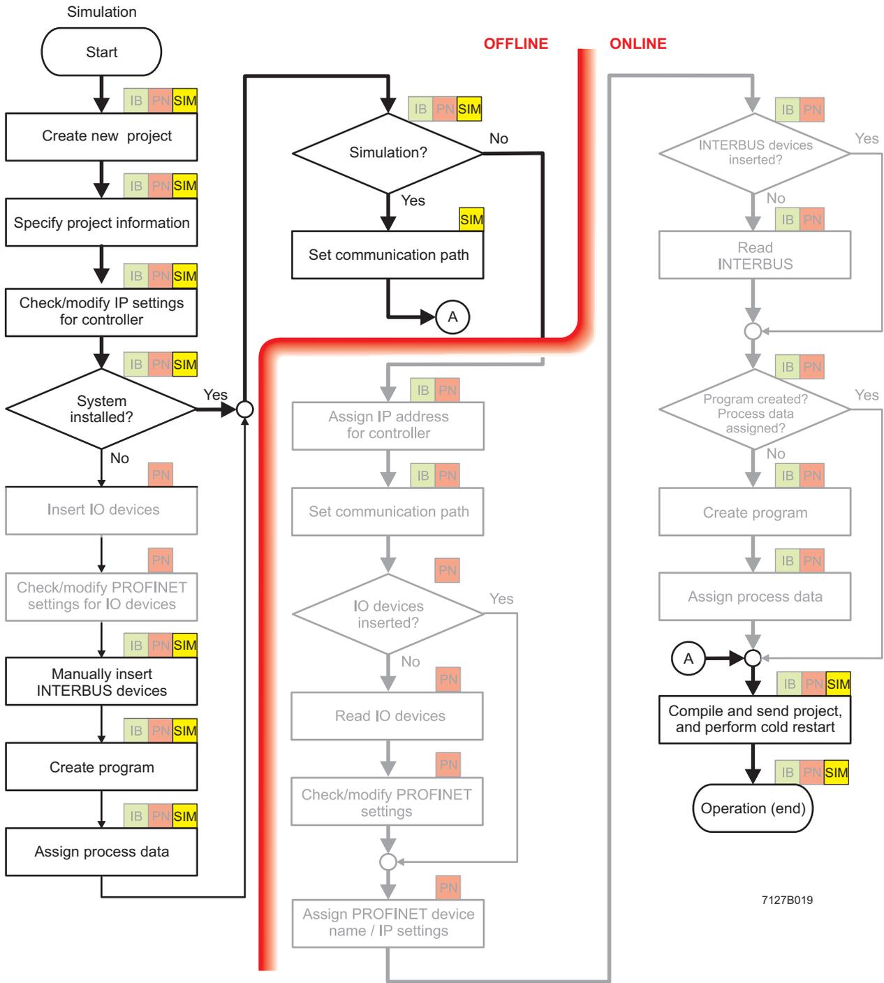
Figure 7-2 Sequence for creating the simulation project
