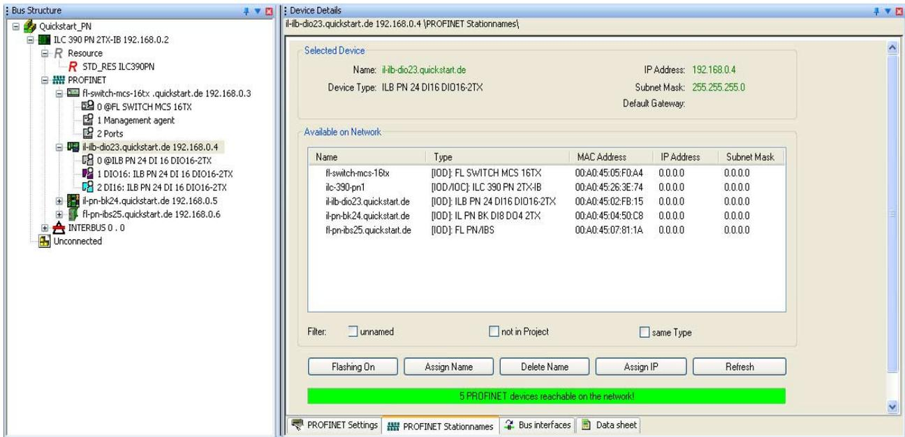
Figure 6-8 List of all PROFINET IO devices that can be accessed in the network
