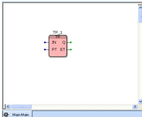
Figure 8-3 Function block in the IEC programming workspace
