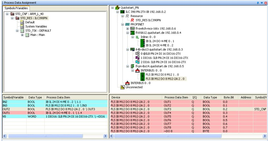
Figure 4-24 All used process data assigned to variables
