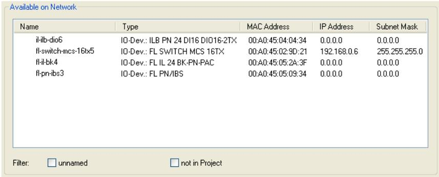
Figure 4-40 Example: All devices with PROFINET device names
