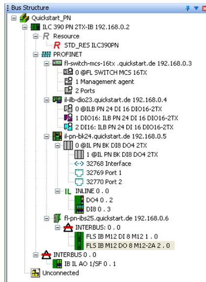
Figure 6-4 Complete bus configuration for the example project
