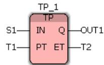
Figure 8-6 TP\_1 function block with all parameters
