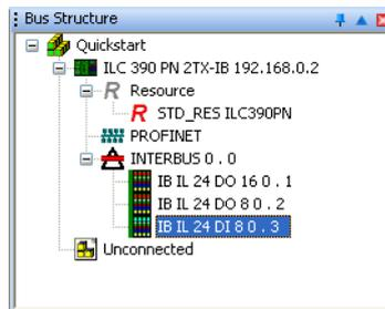
Figure 5-3 Complete bus configuration for the example project
