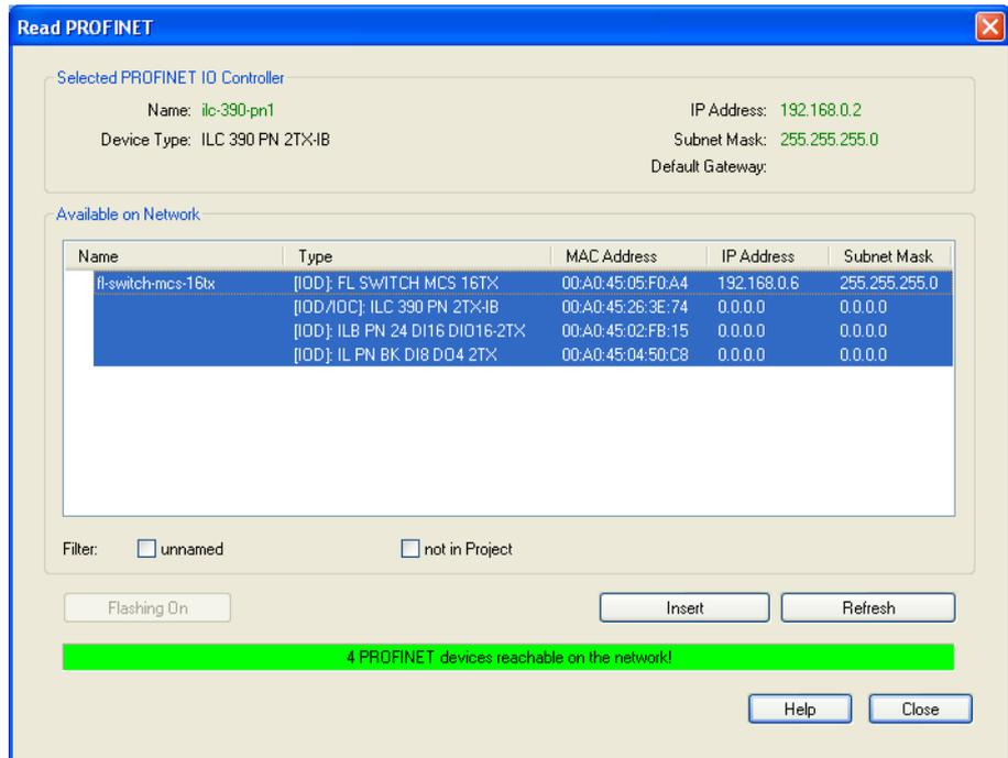
Figure 4-35 Connected and selected PROFINET IO devices for the project; without PROFINET device names and IP addresses
