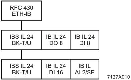
Figure 4-13 Simple bus configuration
