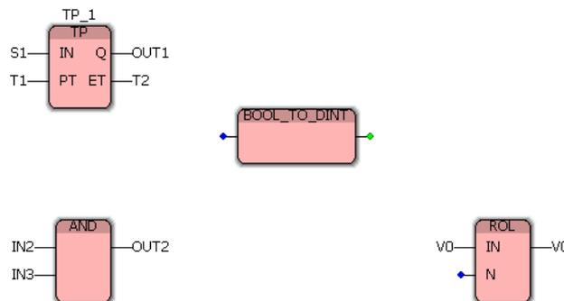
Figure 8-7 All function blocks inserted with the required parameters
