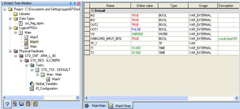
Figure 4-60 Variables in debug mode: Global variables (VAR\_EXTERNAL)
