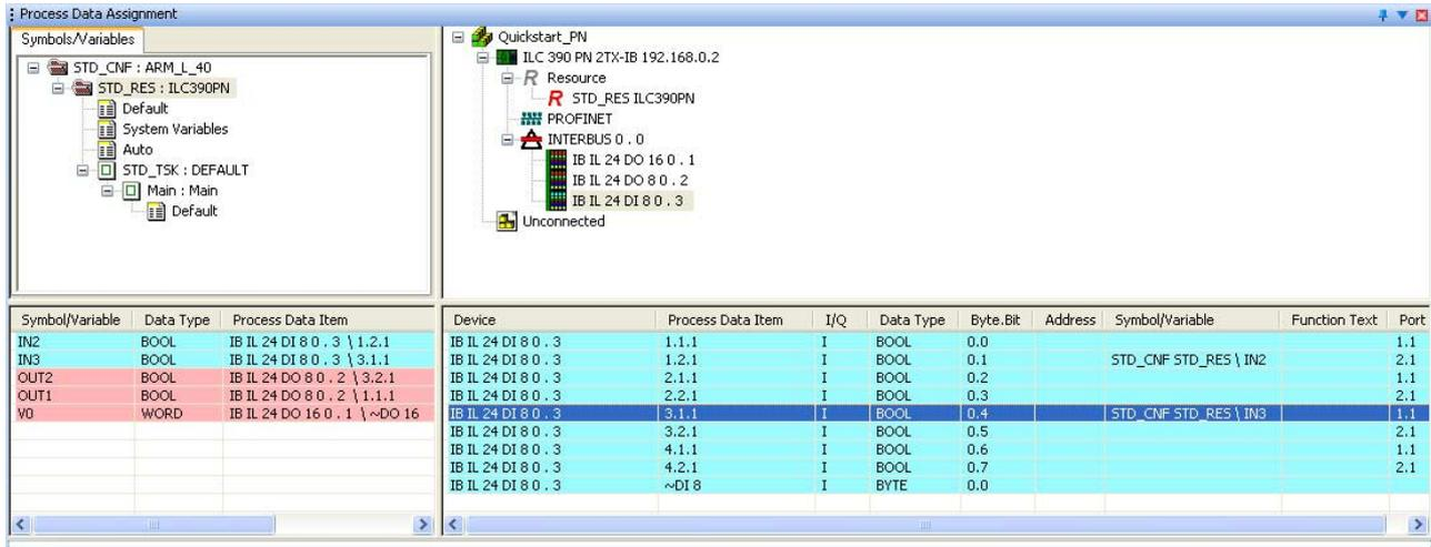
Figure 5-4 All used process data assigned to variables
