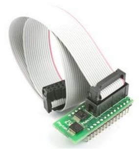
DIP28/BH16 specialized adapter for in system programming of TI MSP430 microcontrollers in JTAG modes.
