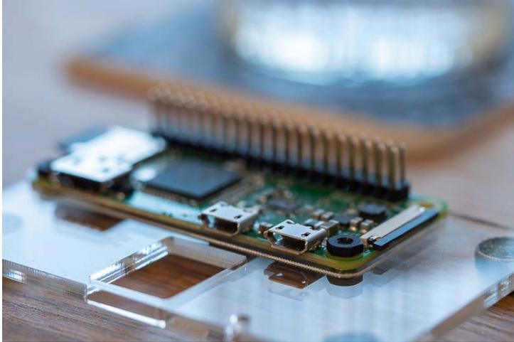
The thinner acrylic piece is a shim layer that levels up the metal standoffs that attach the Keybow PCB to the baseplate and Zero WH, so that they all sit at the same height. We'll fit it now, using one of the standoffs.
