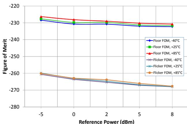
Typical Performance Data @ 25°C,  $V_{DD} = 2.8V$ ,  $f_C = 50$  MHz and  $F_{IN} = 3$  GHz, unless otherwise noted
