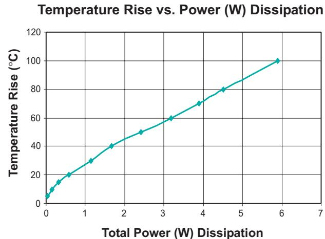
Total Power Dissipation = Copper Loss (W) + Core Loss (W)
