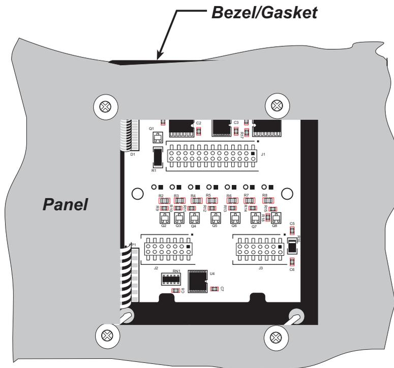
**Figure C-9. LCD/Keypad Module Mounted in Panel (rear view)**
