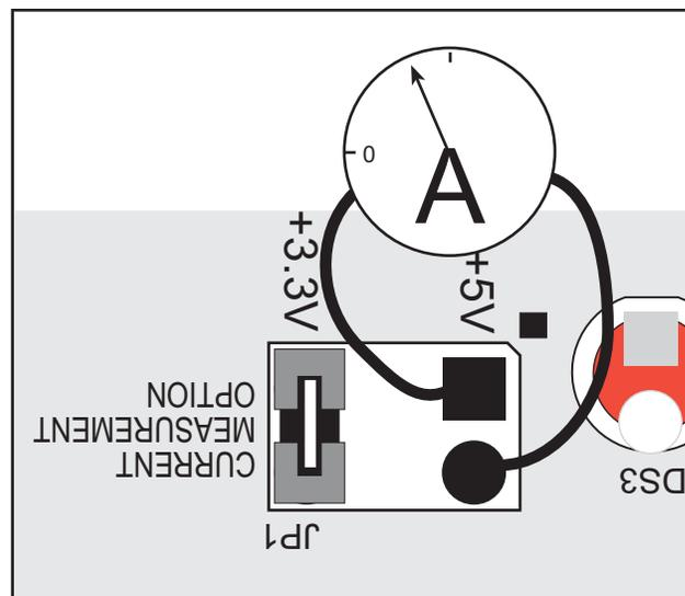
**Figure B-5. Prototyping Board Current-Measurement Option**
