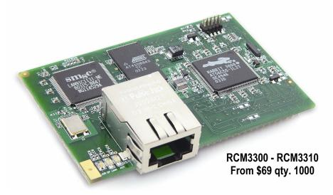
The RCM3300 and RCM3310 come fully loaded: Rabbit 3000 @ 44 MHz clock. 10/100Base-T Ethernet connectivity, 512K Flash, 512K program execution SRAM, 512K data SRAM and up to 50 digital I/O shared with up to 6 serial ports operating at 3.3 V (with 5 V-tolerant I/O). Derived from industrial client feedback combining traditional RabbitCore product strengths into one device, RCM3300 the series microprocessor core modules to
