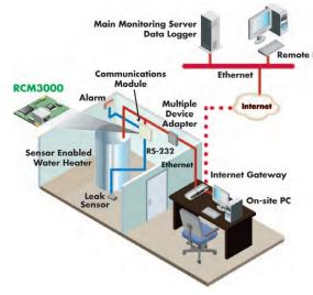
**Potential Applications:** Serial to Ethernet conversion, device web server applications, Ethernet connectivity with I/O and intelligence, device monitoring and data logging.
