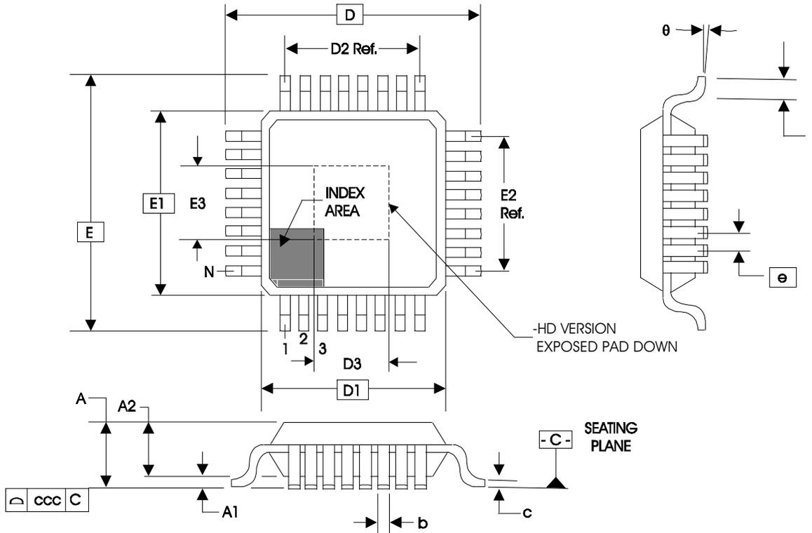
Table 6. Package Dimensions for 64 Lead TQFP, E-Pad
