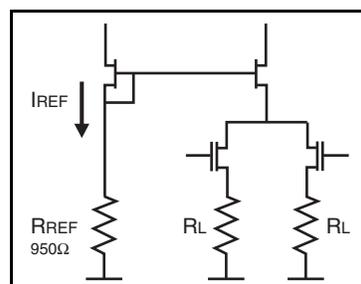
Figure 1. HCSL Current Mirror and Output Drive
