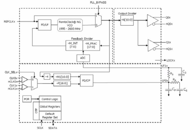
Figure 3. Low Bandwidth Frequency Translator Mode Block Diagram
