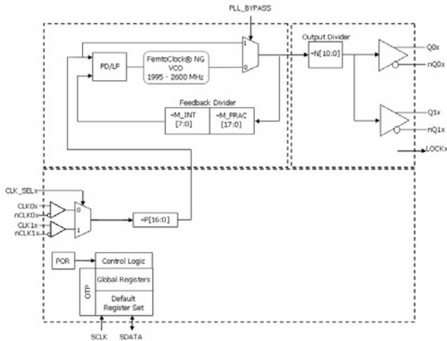
Figure 2. High Bandwidth Frequency Translator Mode Block Diagram
