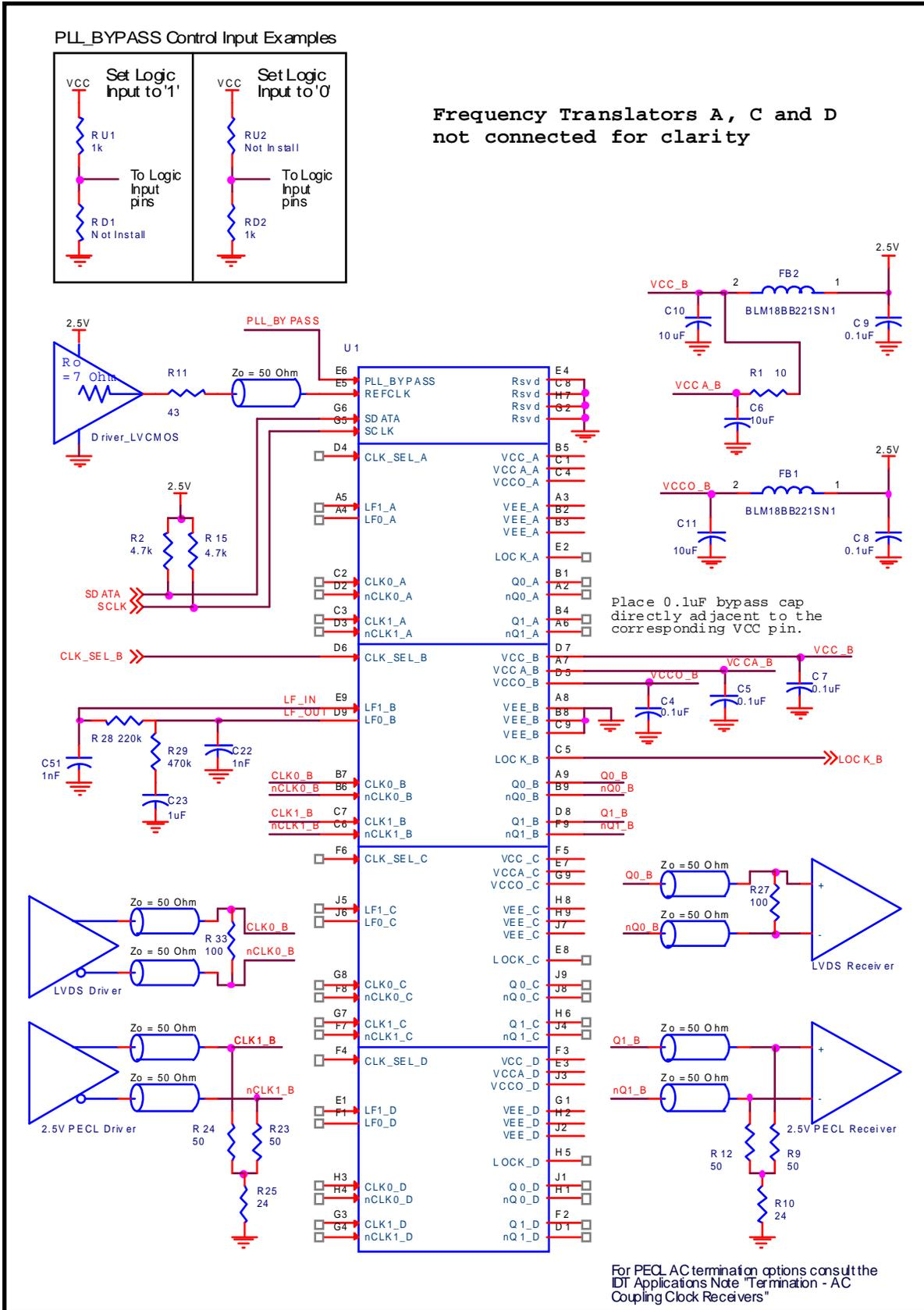
Figure 8. 8T49N488 Schematic Example
