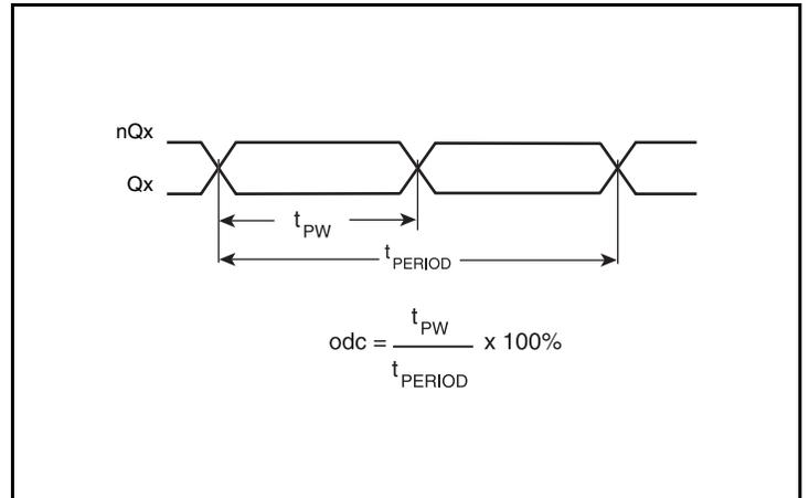
Differential Output Duty Cycle/Output Pulse Width/Period
