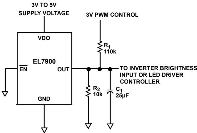
FIGURE 11. AUTOMATIC DIMMING SOLUTION WITH ADJUSTABLE BIAS CONTROL
