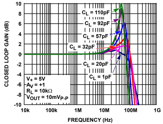
FIGURE 2. GAIN vs FREQUENCY FOR VARIOUS  $C_{LOAD}$
