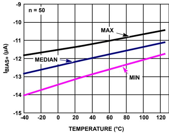
FIGURE 22.  $I_{BIAS+}$  vs TEMPERATURE  $V_S = \pm 2.5V$
