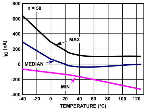
FIGURE 24.  $I_{IO}$  vs TEMPERATURE  $V_S = \pm 2.5V$
