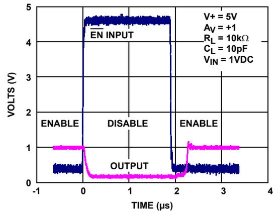
FIGURE 16. ENABLE/DISABLE TIMING
