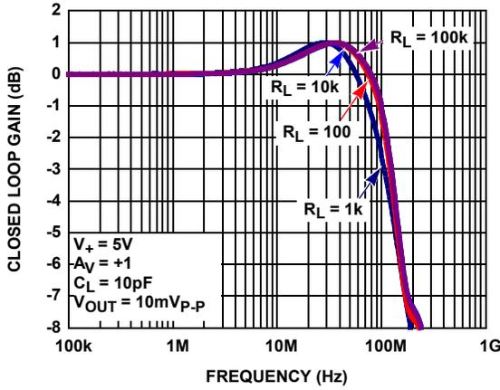
FIGURE 1. GAIN vs FREQUENCY FOR VARIOUS  $R_{LOAD}$
