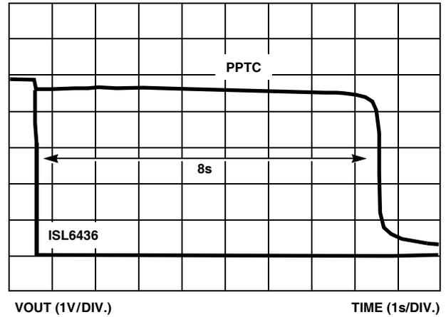
FIGURE 15. ISL6436 vs PPTC WITH EXTENDED 1.5A LOAD
