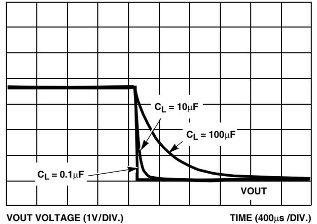
FIGURE 9. FAST TURN -OFF vs  $C_{LOAD}$
