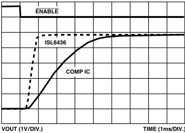
FIGURE 16. COMPARATIVE TURN-ON WAVEFORMS, RI = 10Ω
