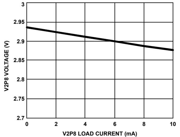
FIGURE 8. V2P8 OUTPUT vs ITS LOAD CURRENT
