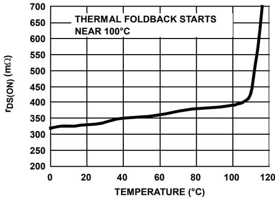
FIGURE 9.  $r_{DS(ON)}$  vs TEMPERATURE AT 3.7V OUTPUT
