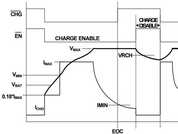
FIGURE 3. TIMING DIAGRAM
