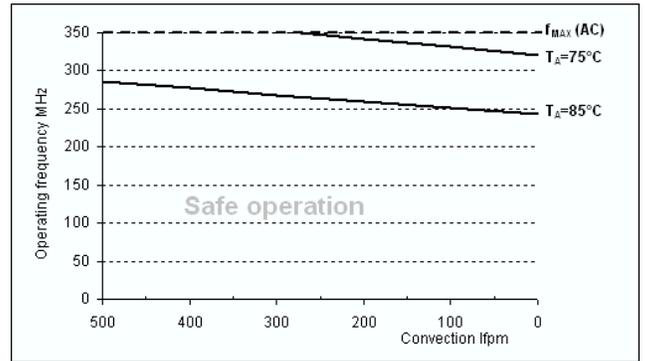
Figure 9. Maximum MPC9443 Frequency, V<sub>CC</sub> = 3.3 V, MTBF 4 Years, 4 pF Load per Line
