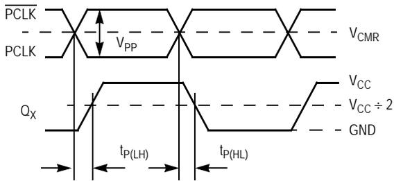
Figure 12. Propagation Delay ( $t_{PD}$ ) Test Reference
