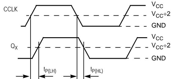
Figure 13. Propagation Delay ( $t_{PD}$ ) Test Reference
