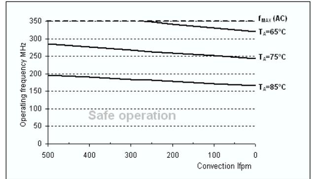
Figure 7. Maximum MPC9443 Frequency, V<sub>CC</sub> = 3.3 V, MTBF 9.1 Years, 4 pF Load per Line
