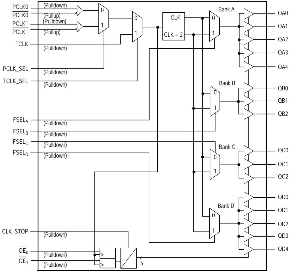
Figure 1. MPC9443 Logic Diagram
