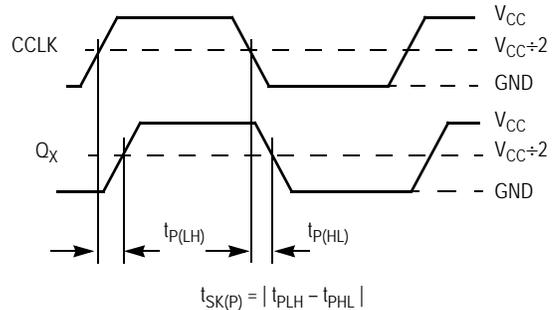
Figure 15. Output Pulse Skew ( $t_{SK(P)}$ ) Test Reference
