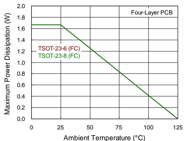
Figure 8. Derating Curve of Maximum Power Dissipation
