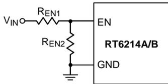
Figure 4. Resistor Divider for Lockout Threshold Setting
