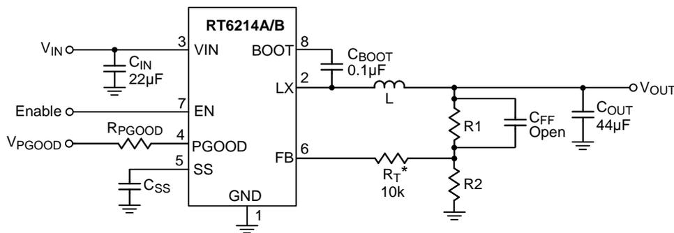
\* Note : When  $C_{FF}$  is added, it is necessary to add  $R_T = 10k$  between feedback network and chip FB pin.
