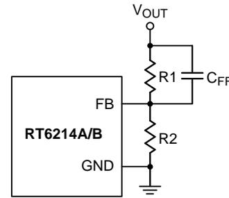
Figure 1. C<sub>FF</sub> Capacitor Setting
