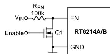
Figure 3. Digital Enable Control Circuit
