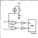
Fig. 14 External circuit for master preset at start-up.
