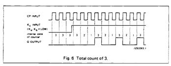
If the "master preset" mode is started two clock cycles or less before an output puise, the output puise will appear at the correct moment. When the output puise appears and the "master preset" mode is not selected, the counter is preset according to the states of the JAM inputs.
