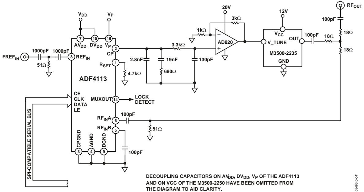
Figure 36. Wideband Phase-Locked Loop
