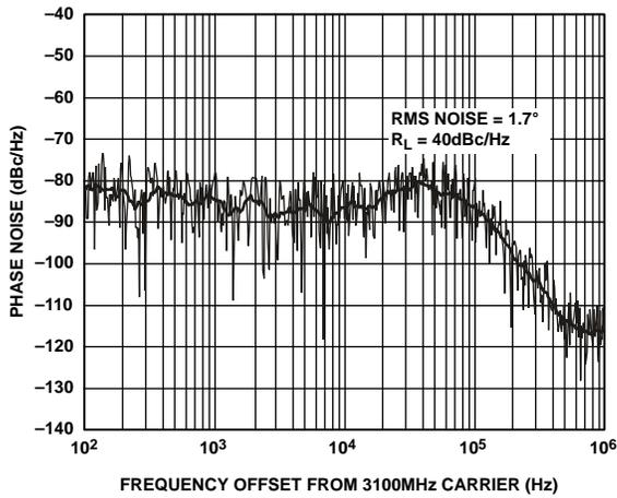
Figure 17. ADF4113 Integrated Phase Noise (3100 MHz, 1 MHz, 100 kHz)
