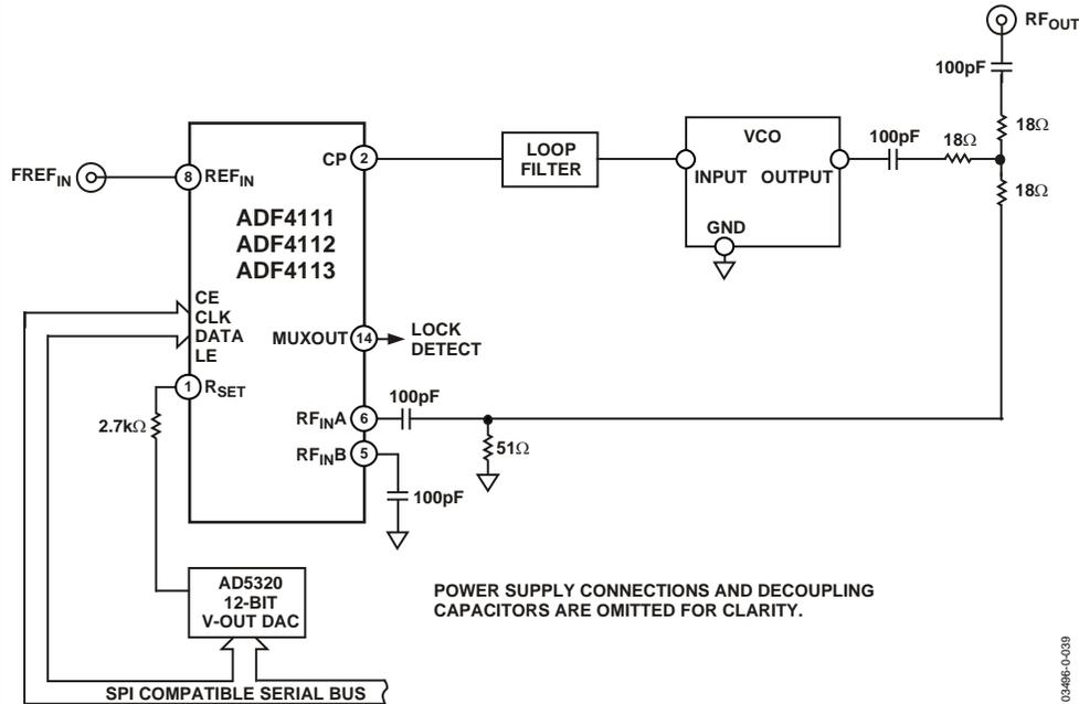
Figure 34. Driving the R<sub>SET</sub> Pin with a D/A Converter
