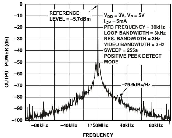
Figure 15. ADF4113 Reference Spurs (1750 MHz, 30 kHz, 3 kHz)
