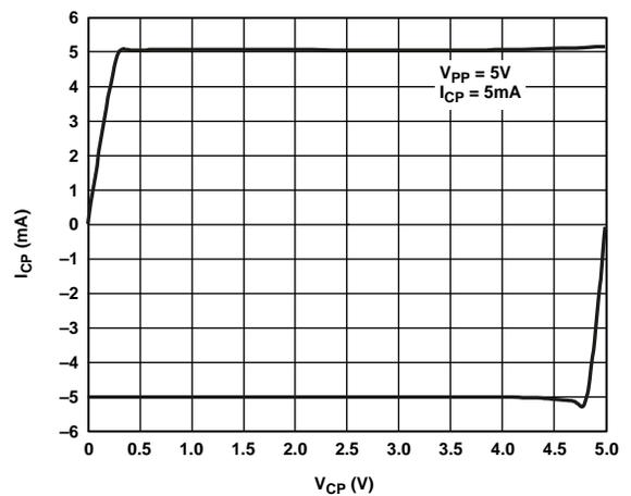
Figure 27. Charge Pump Output Characteristics for ADF4110 Family
