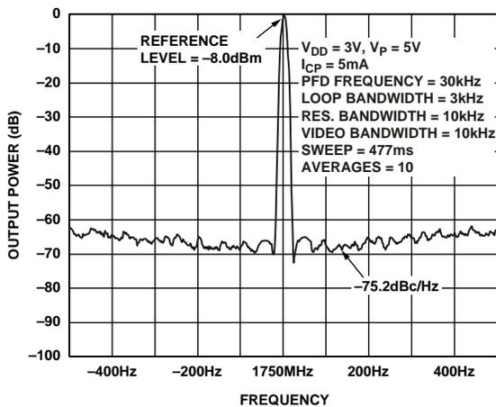
Figure 13. ADF4113 Phase Noise (1750 MHz, 30 kHz, 3 kHz)
