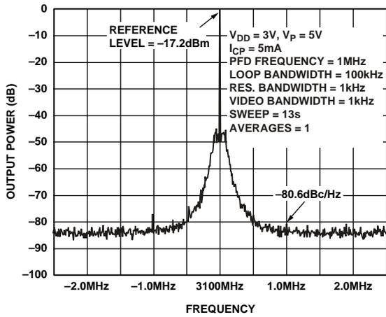
Figure 18. Reference Spurs (3100 MHz, 1 MHz, 100 kHz)
