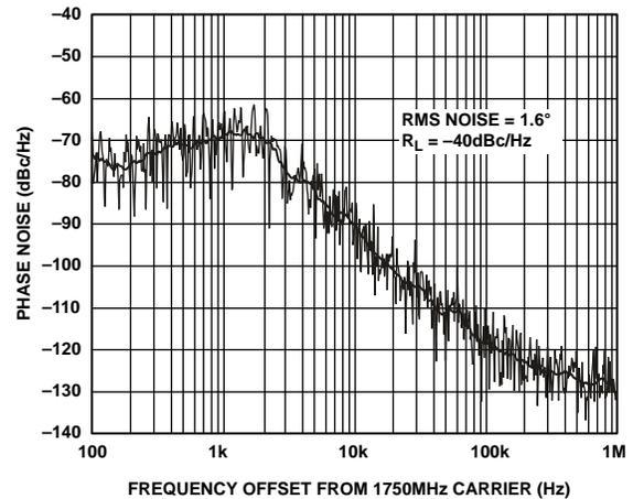
Figure 14. ADF4113 Integrated Phase Noise (1750 MHz, 30 kHz, 3 kHz)
