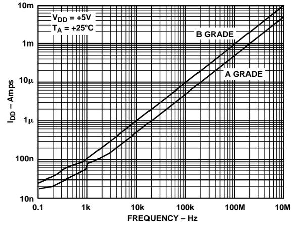
Figure 10. Supply Current vs. Input Switching Frequency
