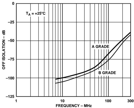
Figure 9. Off Isolation vs. Frequency for Both Grades
