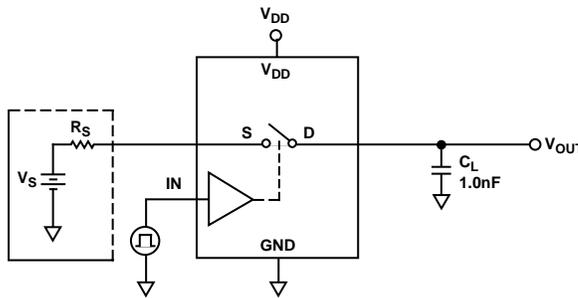
Test Circuit 5. Charge Injection
