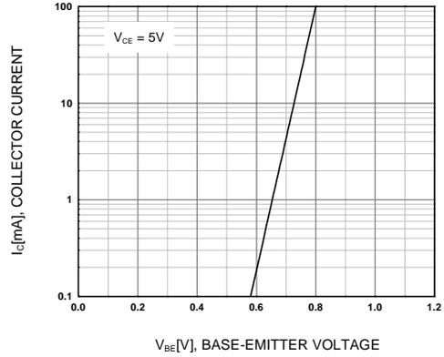
Figure 2. Transfer Characteristic
