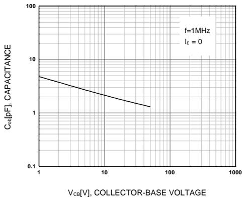
Figure 5. Output Capacitance
