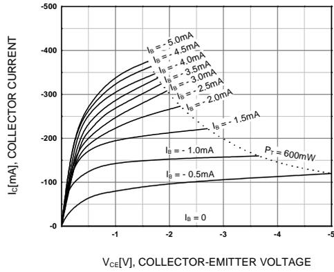
Figure 1. Static Characteristic
