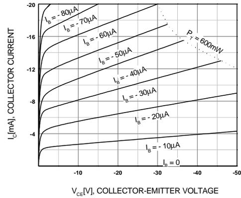
Figure 2. Static Characteristic
