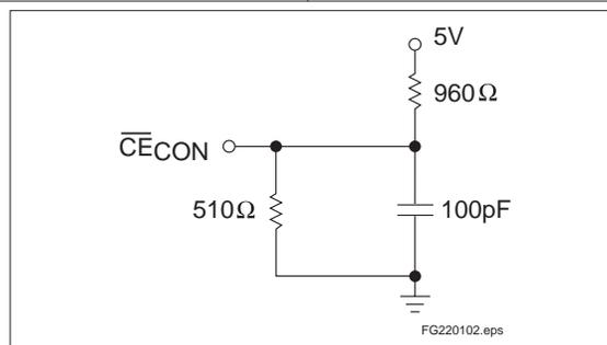
Figure 3. Output Load
