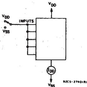
Fig. 10 - Quiescent device current test circuit.
