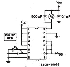
Fig. 9 - Dynamic power dissipation test circuit.
