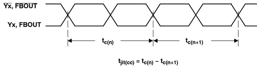
**Figure 3. Cycle-to-Cycle Jitter**
