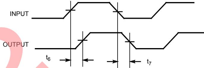
Figure 6. SDRAM Buffer Enable and Disable Times
