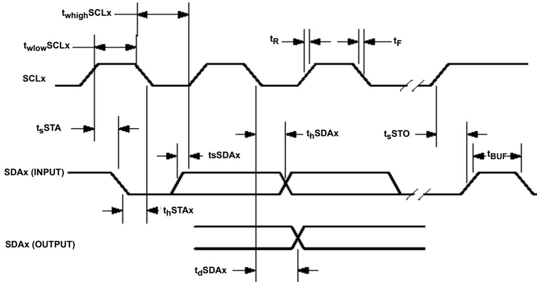
FIGURE 2. I<sup>2</sup>C INTERFACE TIMING
