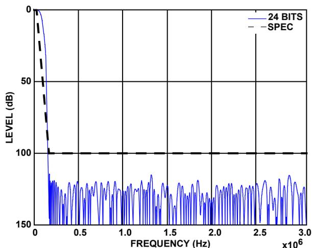
FIGURE 6. ADC DECIMATOR FREQUENCY RESPONSE (256 TAPS DECIMATE BY 32)
