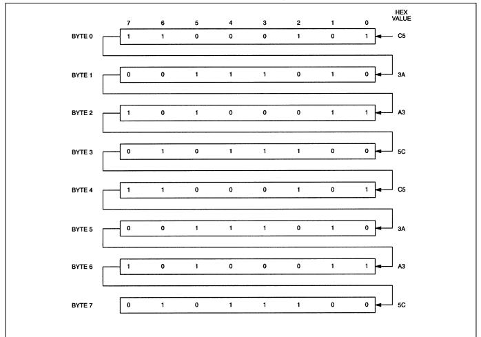
**NOTE**: THE PATTERN RECOGNITION IN HEX IS C5, 3A, A3, 5C, C5, 3A, A3, 5C. THE ODDS OF THIS PATTERN BEING ACCIDENTALLY DUPLICATED AND CAUSING INADVERTENT ENTRY TO THE PHANTOM CLOCK IS LESS THAN 1 IN  $10^{19}$ . THIS PATTERN IS SENT TO THE PHANTOM CLOCK LSB TO MSB.
