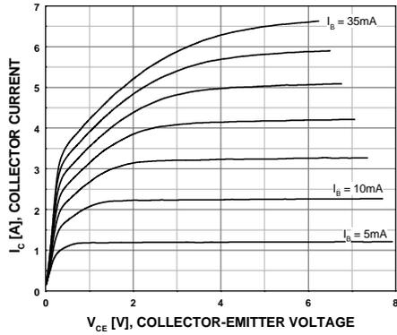
Figure 1. Static Characteristic
