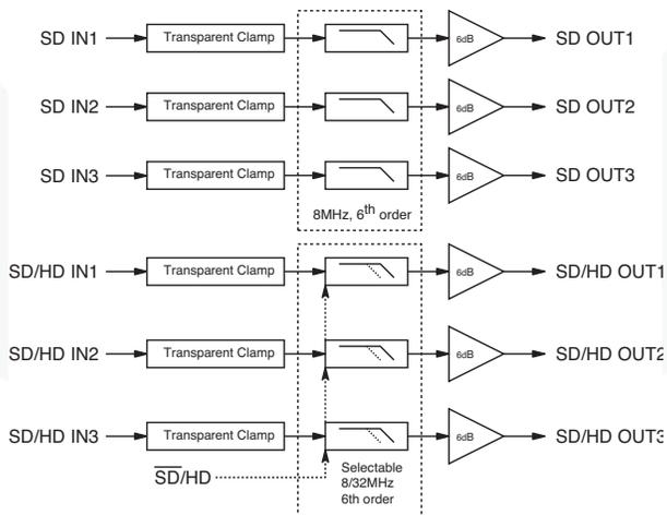
Figure 1. Block Diagram
