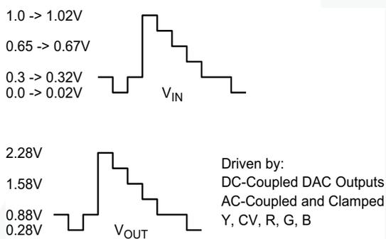
There is a 280mV offset from the DC input level to the DC output level.  $V_{OUT} = 2 * V_{IN} + 280mV$ .
