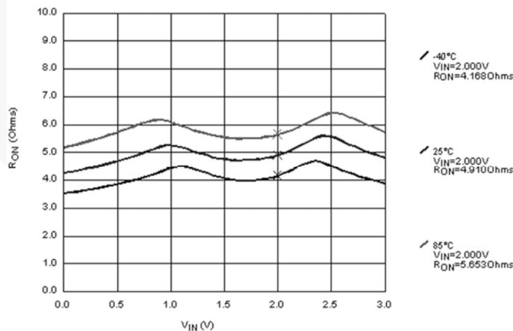
Figure 10. R<sub>ON</sub> Switch On Resistance, I<sub>ON</sub>=26mA, V<sub>CC</sub>=3.0V
