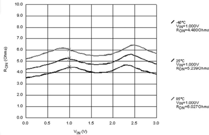
Figure 9. R<sub>ON</sub> Switch On Resistance, I<sub>ON</sub>=13mA, V<sub>CC</sub>=3.0V
