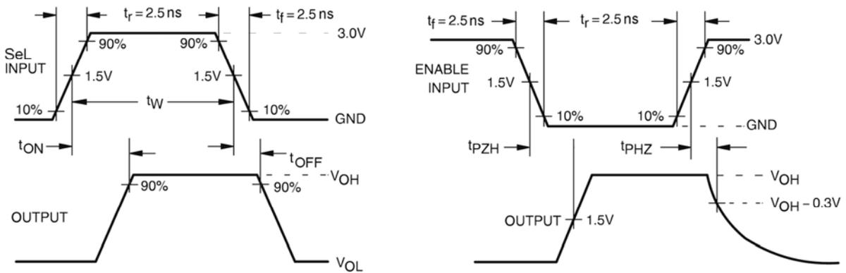
**Figure 12. AC Waveforms**
