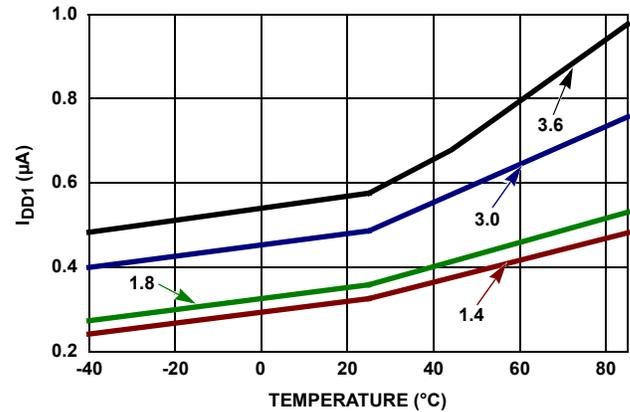
FIGURE 3. I<sub>DD1</sub> vs TEMPERATURE
