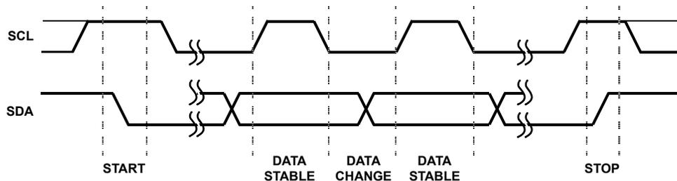
FIGURE 5. VALID DATA CHANGES, START, AND STOP CONDITIONS
