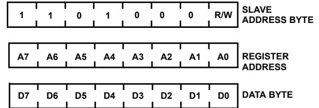
FIGURE 8. SLAVE ADDRESS, WORD ADDRESS, AND DATA BYTES
