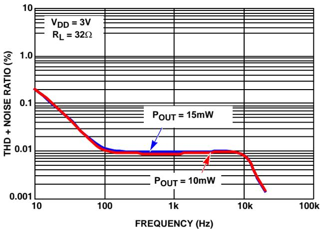
FIGURE 7. TOTAL HARMONIC DISTORTION + NOISE RATIO vs FREQUENCY
