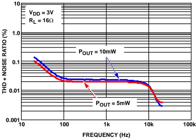
FIGURE 5. TOTAL HARMONIC DISTORTION + NOISE RATIO vs FREQUENCY
