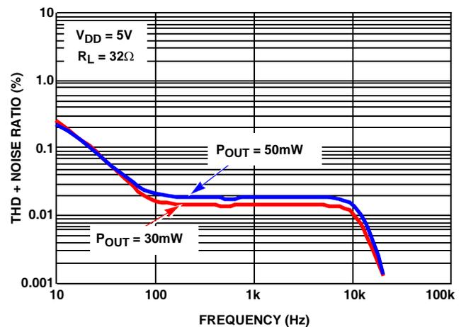
FIGURE 8. TOTAL HARMONIC DISTORTION + NOISE RATIO vs FREQUENCY
