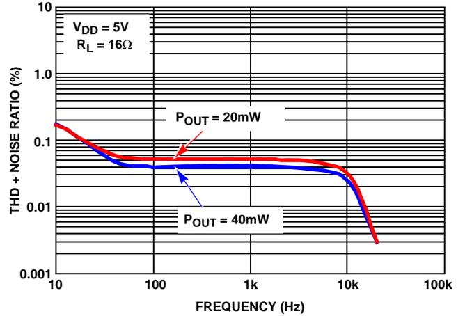
FIGURE 6. TOTAL HARMONIC DISTORTION + NOISE RATIO vs FREQUENCY
