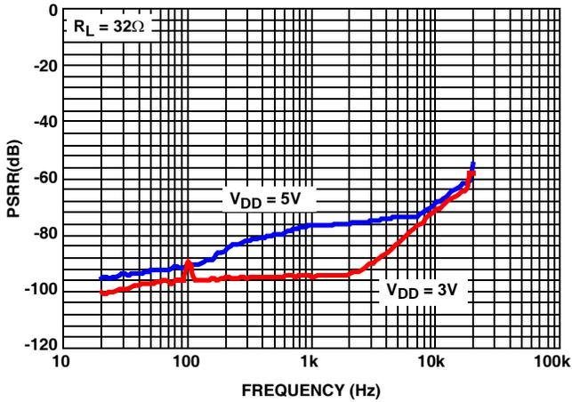
FIGURE 9. POWER SUPPLY REJECTION RATIO vs FREQUENCY
