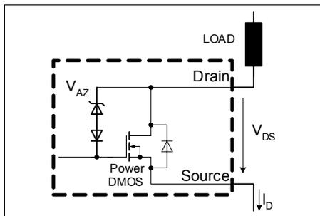
**Figure 7 Inductive and Over voltage Output Clamp**
