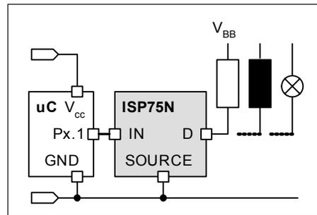
**Figure 8 Application Circuit**
