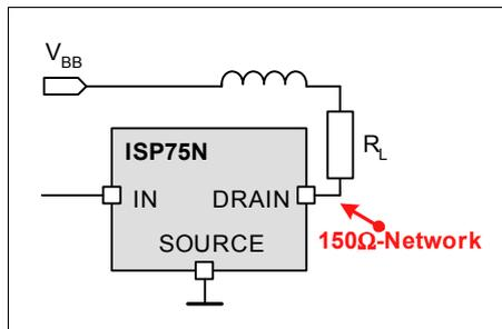
Figure 4 Test circuit for conducted emission <sup>1)</sup>
