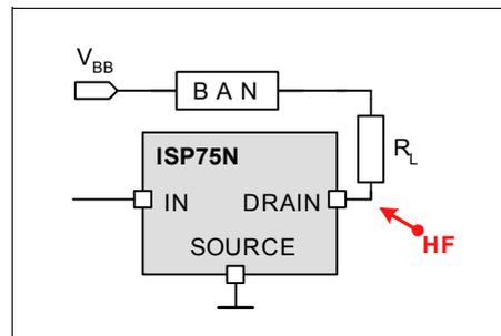
Test circuit for conducted susceptibility <sup>2)</sup>
