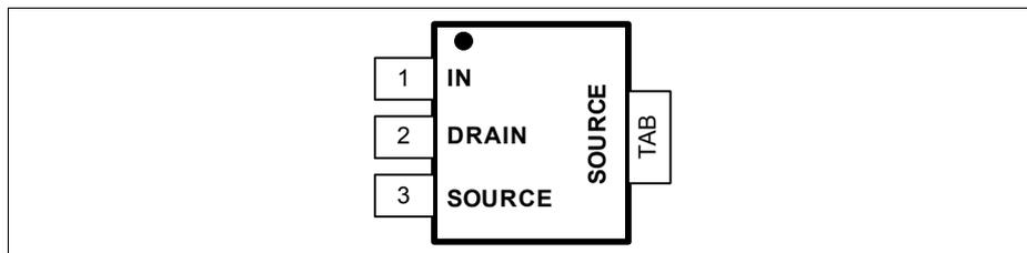
Figure 2 Pin Configuration
