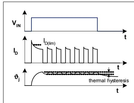
Figure 11 Short circuit
