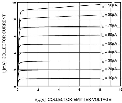
Figure 1. Static Characteristic
