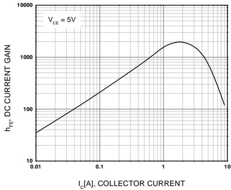
Figure 1. Static Characteristic
