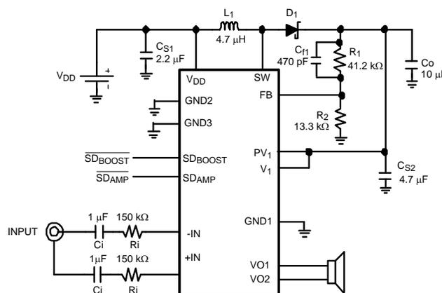
**Figure 1. Typical LM48510 Audio Amplifier Application Circuit**
