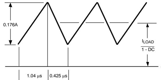
**Figure 29. 10 $\mu$ H Inductor Current
