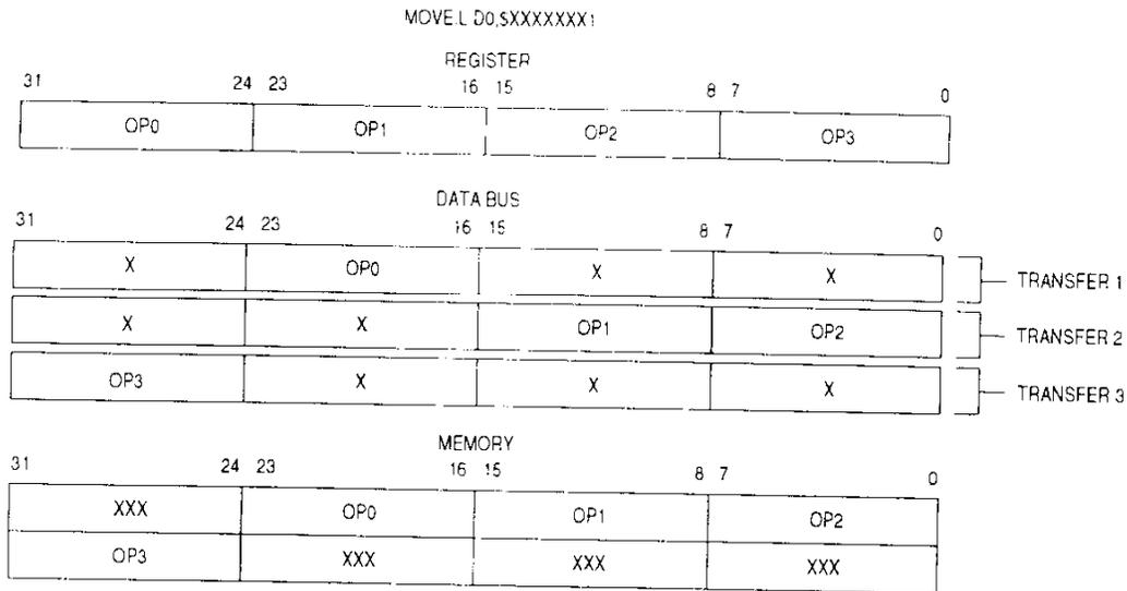
Figure 7-9. Example of a Misaligned Long-Word Transfer
