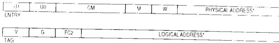
\*FOR 4-KBYTE PAGE SIZES, THIS FIELD USES ADDRESS BITS 31-12; FOR 8-KBYTE PAGE SIZES, BITS 31-13
