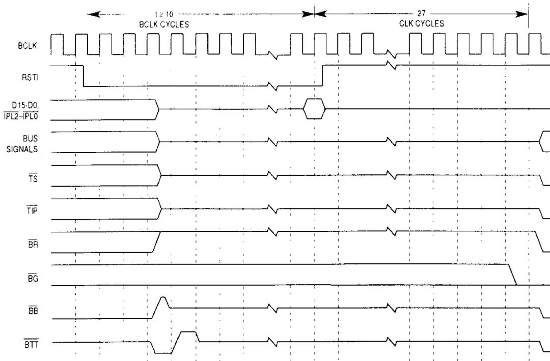
NOTE: For the processor to reset begin bus cycles after reset,  $\overline{BG}$  must be asserted,  $\overline{TS}$  must be negated or pulled up.  $\overline{BTT}$  must be asserted (or  $\overline{BTT}$  transition from asserted to negated) eventually to indicate an end to the alternate master's tenure.
