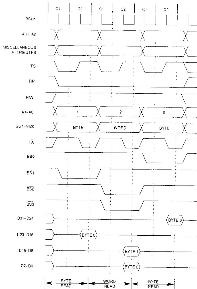
Figure 7-11. Misaligned Long-Word Read Bus Cycle Timing
