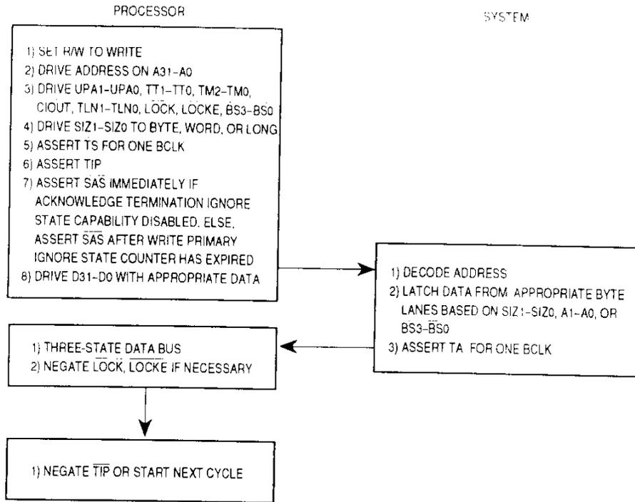
Figure 7-18. Byte, Word, and Long-Word Write Transfer Flowchart
