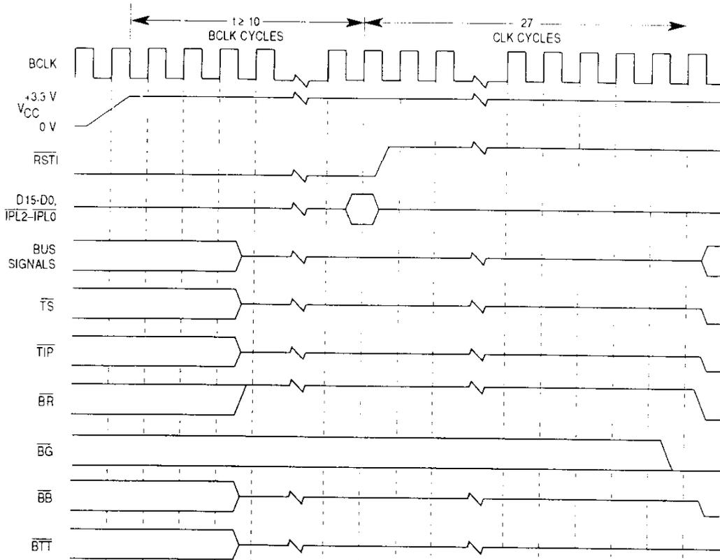
NOTE: For the processor to begin bus cycles after reset,  $\overline{BG}$  must be asserted,  $\overline{TS}$  must be negated or pulled up. If bus arbitration activity is started by an alternate master ( $\overline{TS}$  asserted),  $\overline{BTI}$  must be asserted (or  $\overline{BB}$  transition from asserted to negated) eventually to indicate an end to the alternate master's tenure.
