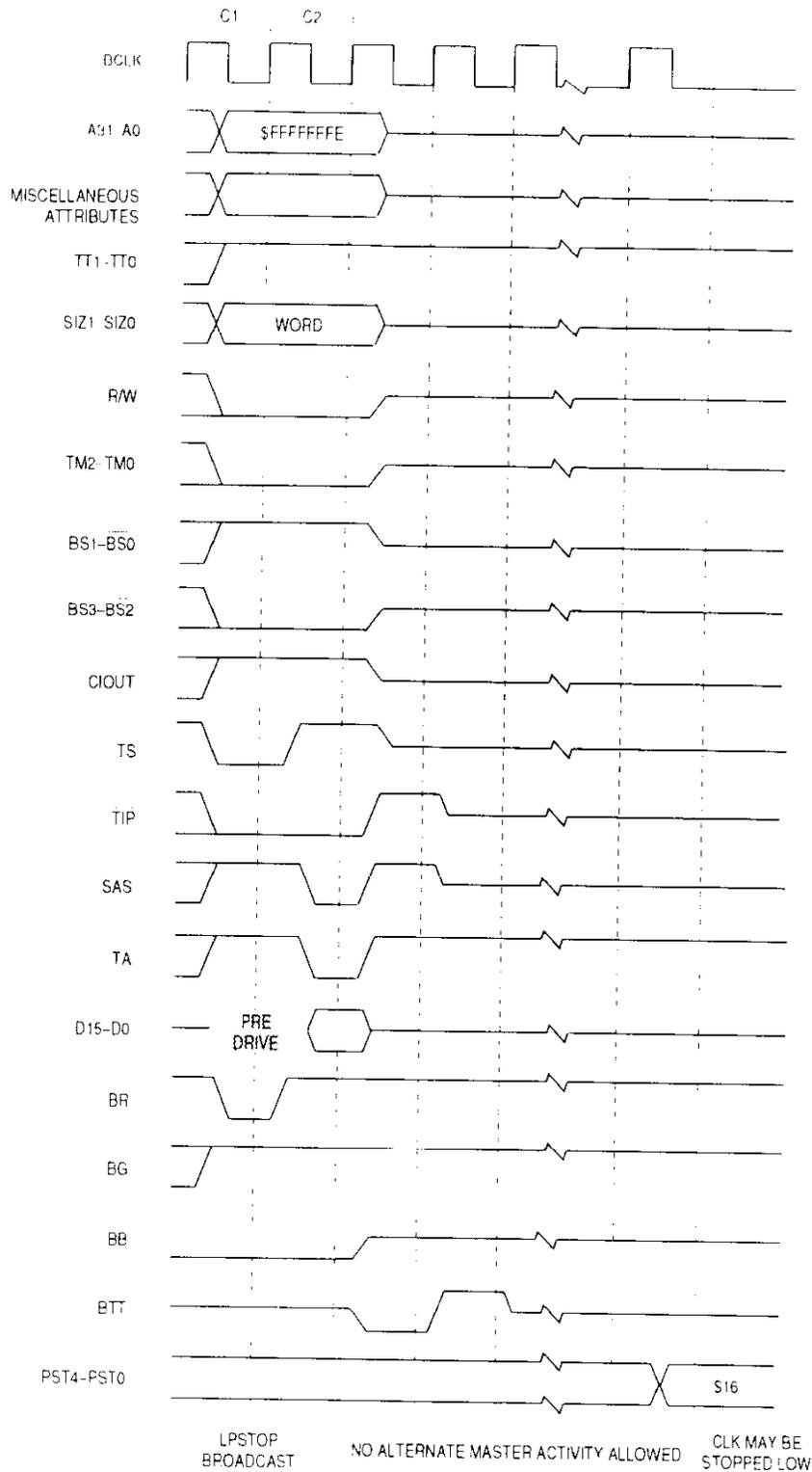
Figure 7-33. LPSTOP Broadcast Bus Cycle Timing,  $\overline{BG}$  Negated
