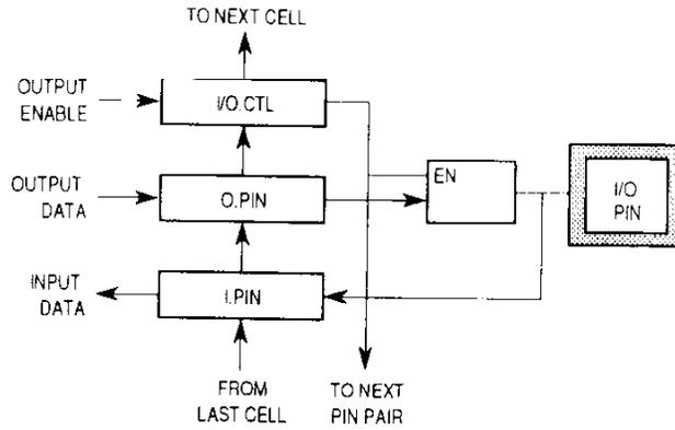
**Figure 9-7. General Arrangement of Bidirectional Pin Cells**
