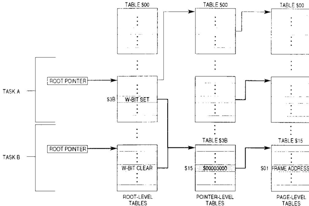
\* PAGE FRAME ADDRESS SHARED BY TASK A AND B; WRITE PROTECTED FROM TASK A.
