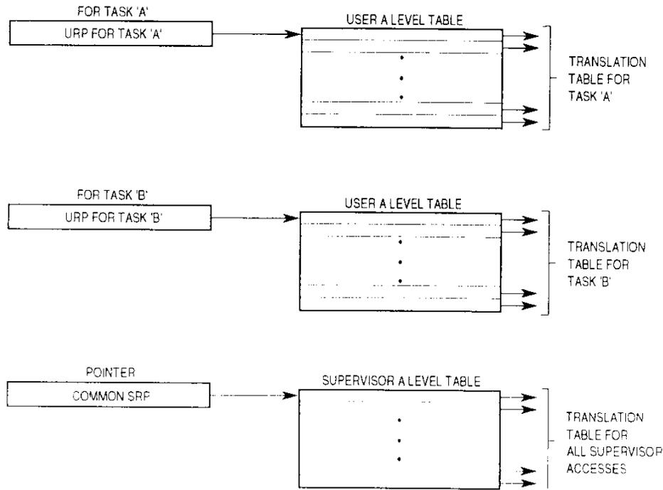
**Figure 4-16. Translation Table Structure for Two Tasks**
