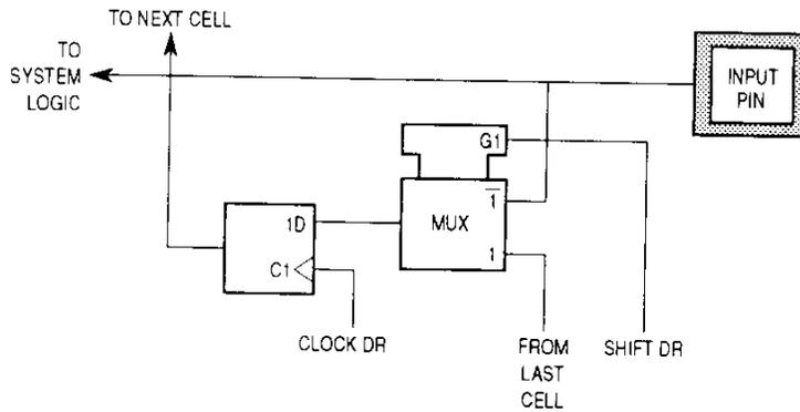
Figure 9-4. Observe-Only Input Pin Cell (I.Obs)
