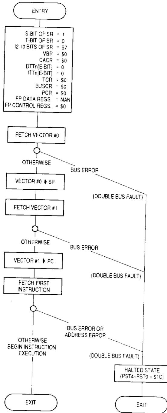
Figure 8-5. Reset Exception Processing Flowchart
