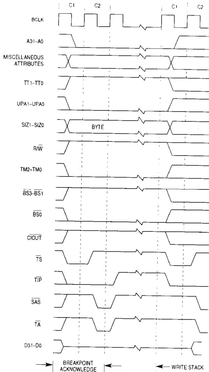
Figure 7-31. Breakpoint Interrupt Acknowledge Bus Cycle Timing
