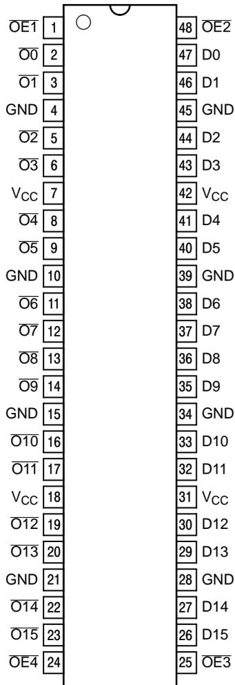
Figure 1. Pinout: TSSOP-48 (Top View)
