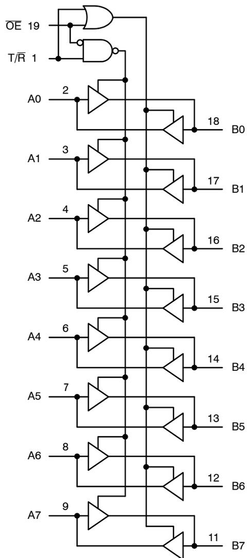
Figure 2. Logic Diagram
