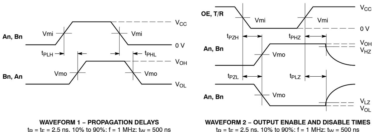
Figure 3. AC Waveforms
