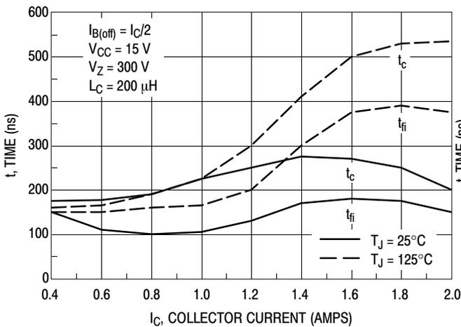
Figure 11. Inductive Switching,  $t_c$  and  $t_{fi}$ ,  $I_C/I_B = 5$
