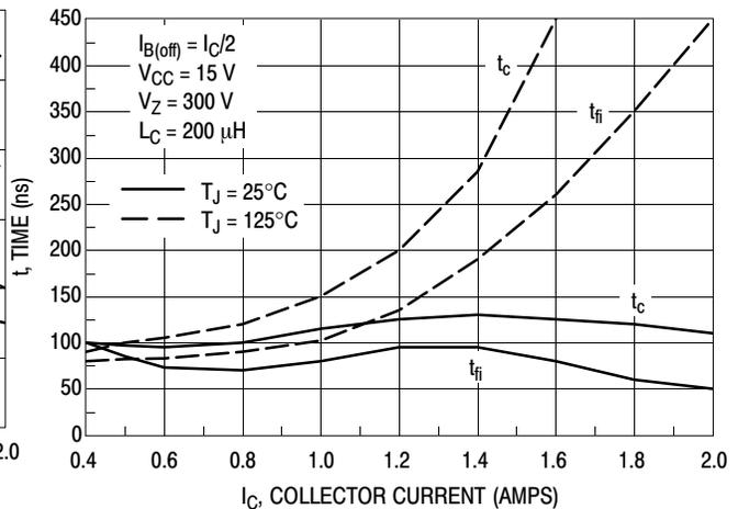
Figure 12. Inductive Switching,  $t_c$  and  $t_{fi}$ ,  $I_C/I_B = 10$
