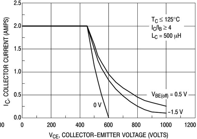
Figure 16. Reverse Bias Switching Safe Operating Area
