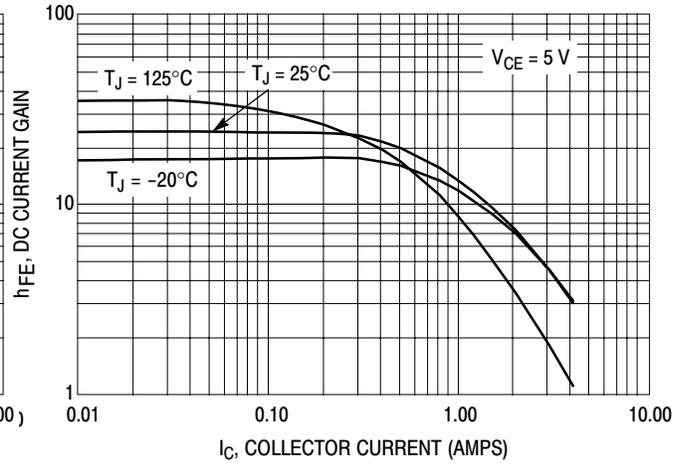
Figure 2. DC Current Gain @ 5 Volts
