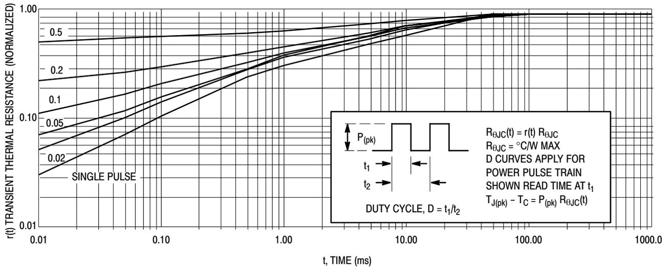
Figure 20. Typical Thermal Response ( $Z_{\theta JC}(t)$ ) for MJE18002
