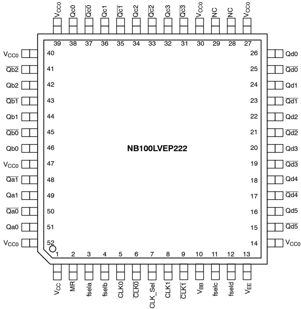
All V<sub>CC</sub>, V<sub>CC0</sub>, and V<sub>EE</sub> pins must be externally connected to appropriate Power Supply to guarantee proper operation. V<sub>CC</sub> pin internally connected to V<sub>CC0</sub> pins. The thermally conductive exposed pad on package bottom (see package case drawing) must be attached to a heat-sinking conduit. This exposed pad is electrically connected to V<sub>EE</sub> internally.
