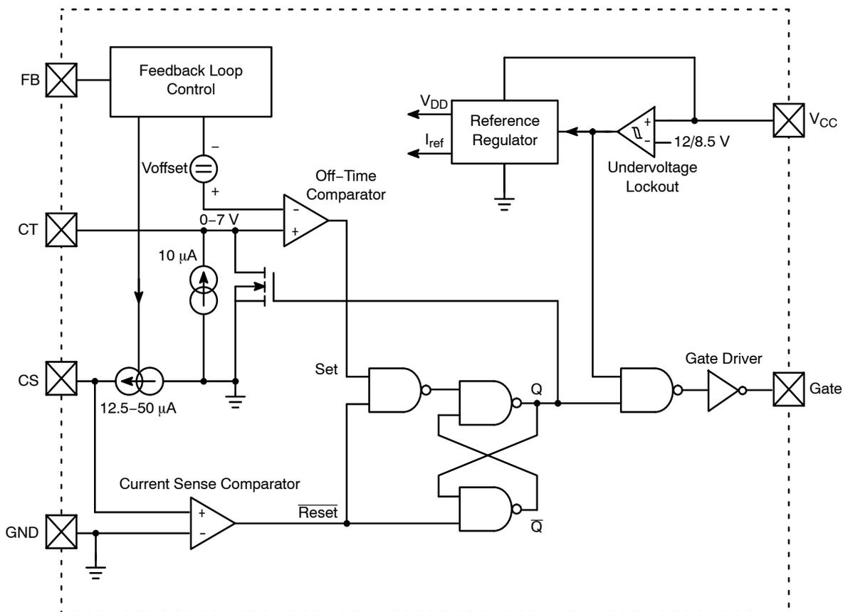
**Figure 2. Representative Block Diagram**
