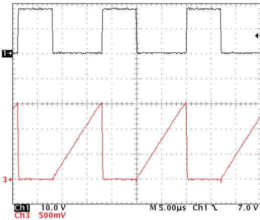
**Figure 22. CT Voltage at Full Load Condition**
