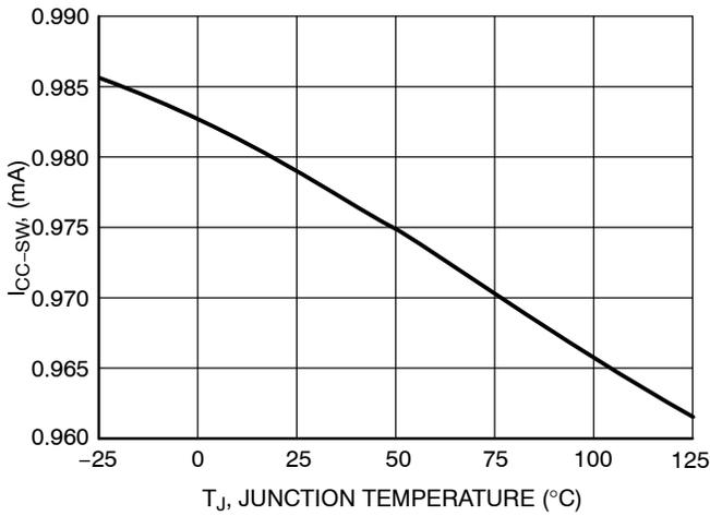
Figure 5. Operating Current Consumption vs. Junction Temperature
