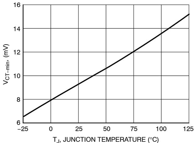
**Figure 10. CT pin Threshold vs. Junction Temperature**
