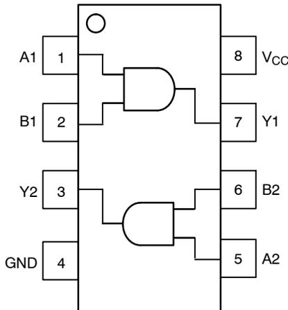
Figure 1. Pinout
