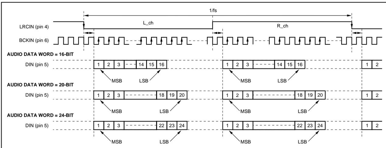
FIGURE 2. "I<sup>2</sup>S" Data Input Timing.
