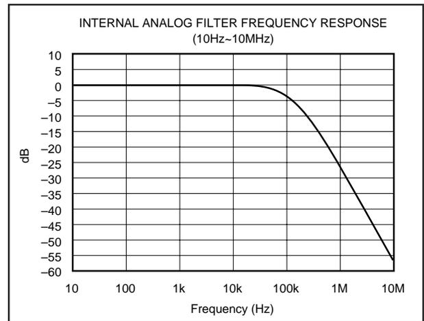
FIGURE 8. Low Pass Filter Wideband Frequency Response.
